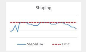
Traffic shaping involves queueing or buffering network packets around the set limit to provide a smooth end-user experience. Excess packets are sent when bandwidth is available. Other measures involve flow-control, where an XOFF signal pauses a sender to avoid contention.
