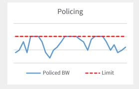
Bandwidth policing with UTMs and routers typically involves dropping packets upon reaching a limit. These devices lack the capacity for more sophisticated shaping controls, resulting in a poor user experience with video streams being reset or buffering continuously.
