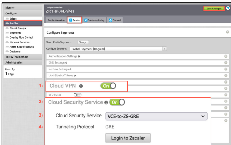
Figure 21. GRE profile for cloud security service
