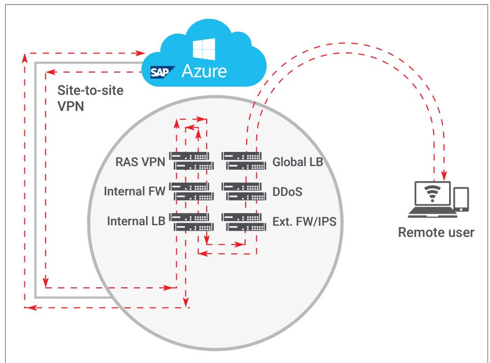
*Internet-bound traffic from remote users takes a slow, circuitous path as it's routed through the data center security stack before it can head out to the cloud or open internet, then goes back through the stack on its return trip.*
